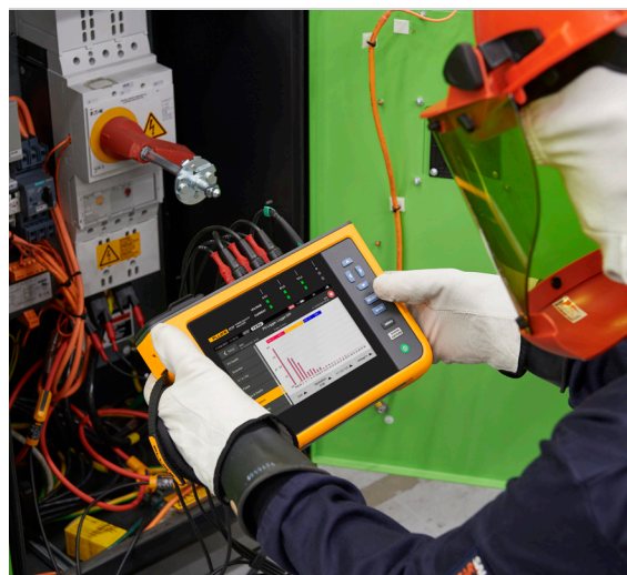
Fluke 1777 driefasen Power Quality Analyzers
